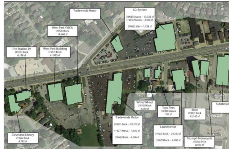
Figure 135. Existing Conditions in the Civic Node and along Lorain Ave. (Viking Planning Group)
